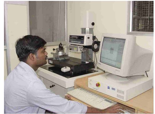
Contour Tracer - highly precise surface contour measurements
