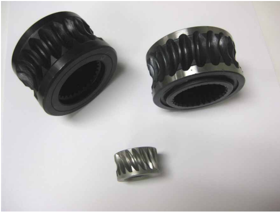
Worm Gears / Wheels of Various Sizes Broached, OD Ground, Heat-treated
